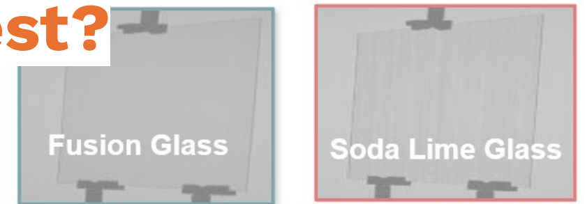
Photos with shadowgraph at 60 degrees tilt
