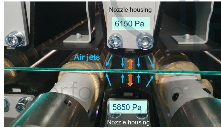
These controls are used to keep glass as flat.
