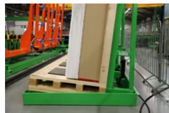
Fig. 3: Hydraulic crate tilter capable of various tilt angles.
