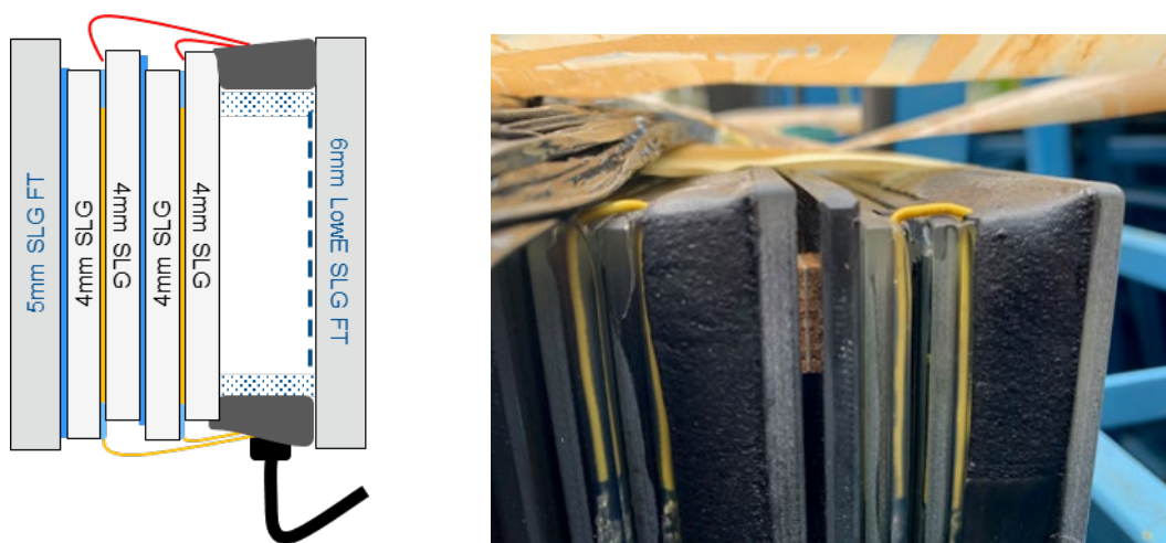
Fig. 5: Schematic and side view of a dynamic smart window.
