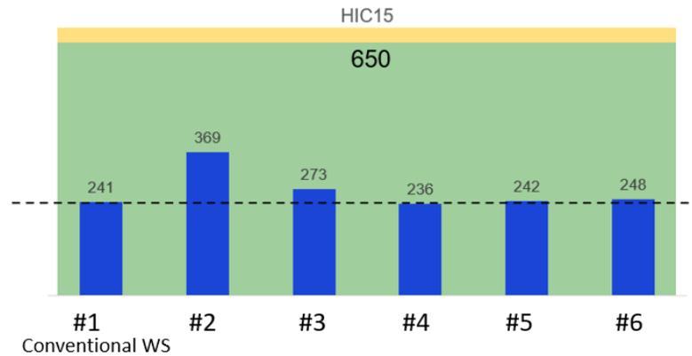
Figure 8. Comparison of HIC values obtained by modeling for 6 laminate options.
