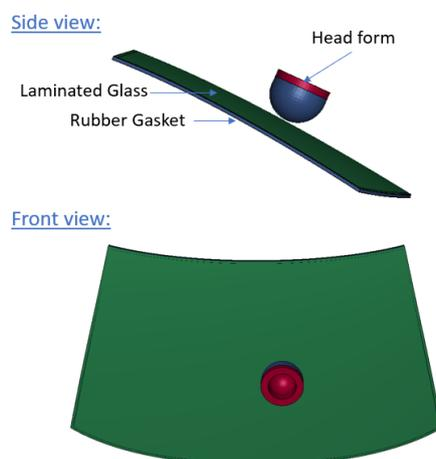
Figure 3. PedPro FE model, side, and front views
