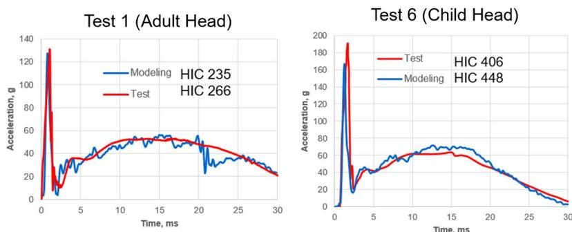
Figure 7. Model validation for different test scenarios: Test results vs. modeling prediction. Acceleration-time curve and HIC values.
