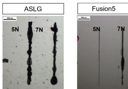
Figure 2. Knoop Scratch Test at 5N and 7N.
