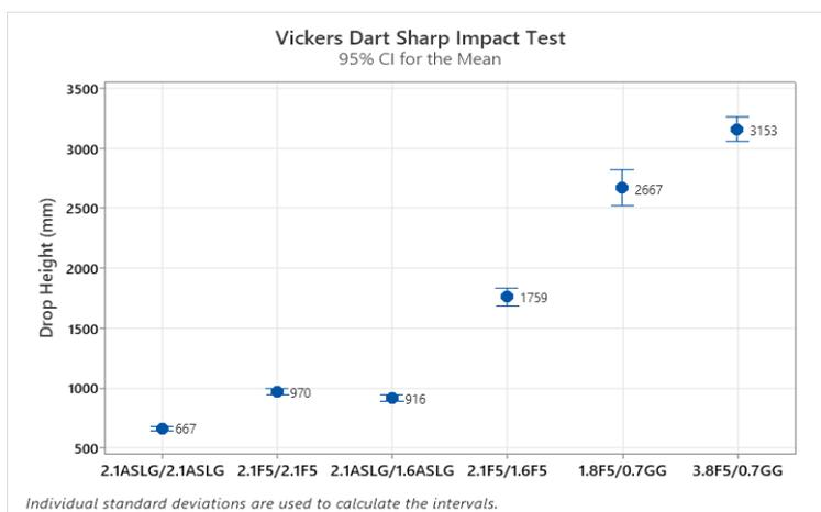
Figure 1. Vickers Dart Drop Test results for traditional SLG laminates vs. laminates with Fusion5® and Corning® Gorilla® Glass. In the plot “ASLG” is “annealed soda-lime glass”, “F5” is “Fusion5®” and “GG” is “Corning® Gorilla® Glass”.
