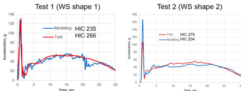
Figure 5. Model validation for different WS shapes: Test results vs. modeling prediction. Acceleration-time curve and HIC values.
