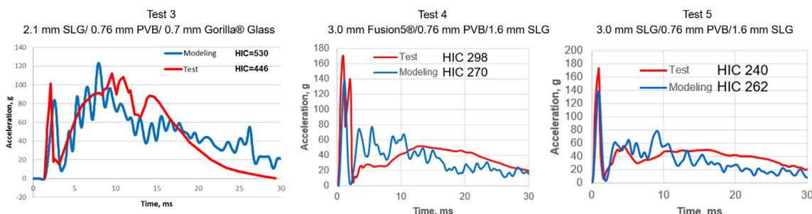
Figure 6. Model validation for different WS constructions: Test results vs. modeling prediction. Acceleration-time curve and HIC values.
