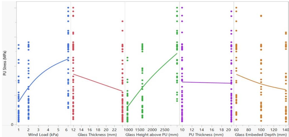
Figure 1: Embedment stress (PU Stress) as a function of each model input.
