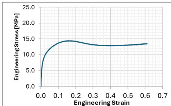
Figure 1: Averaged stress-strain curve for DOWSIL™ 375
