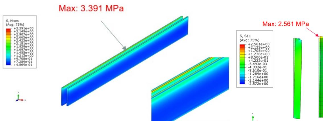
Figure 4: Stress output for a single condition highlighting the stress distribution through the embedment material.
