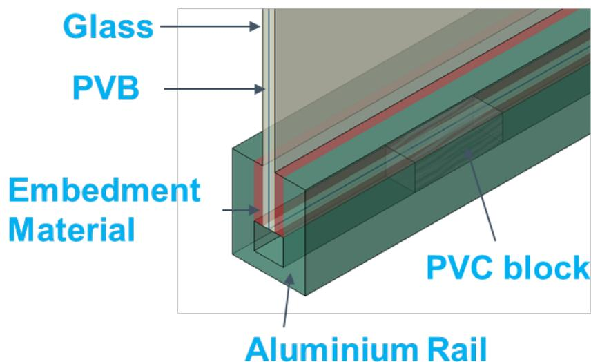
Figure 2: A schematic of the glass embedment system.
