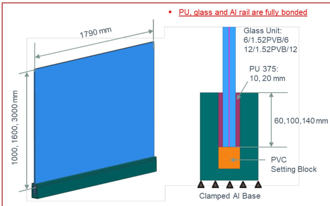
Figure 3:: A schematic of the modelling inputs utilized in the DOE.
