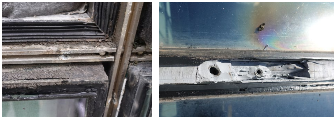
Fig. 10: Crossing point with blocked inner sealing level and destroyed edge bonding (left) and glass rebate filled with silicone and first damage on the coating of the IGU (right).
