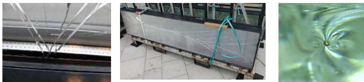
Fig. 9: thermal breakage / climatic load breakage IGU / Spontaneous failure nickel sulphide inclusion.
