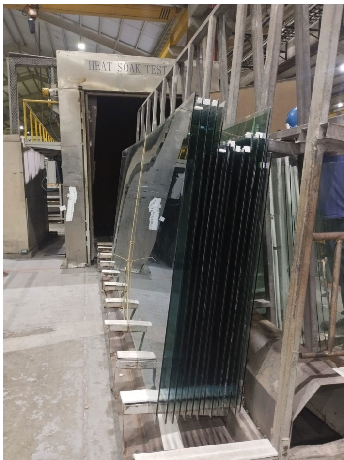
Fig. 4: Glass being loaded to Heat Soak Furnace.
