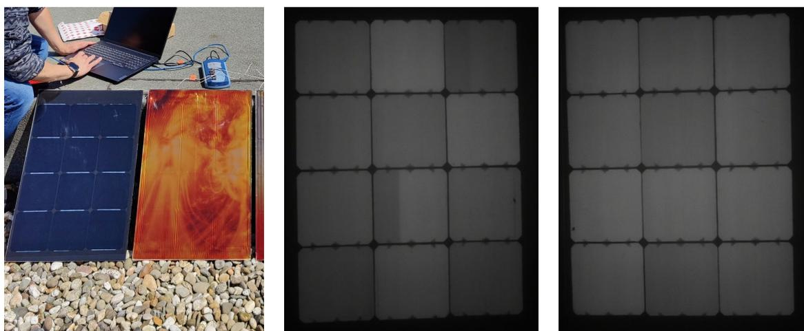
Figure 2: "Photographs of Handmade Laboratory Prototypes" and "EL Imaging Results of Laboratory Modules." ref. module left, colored module right.
