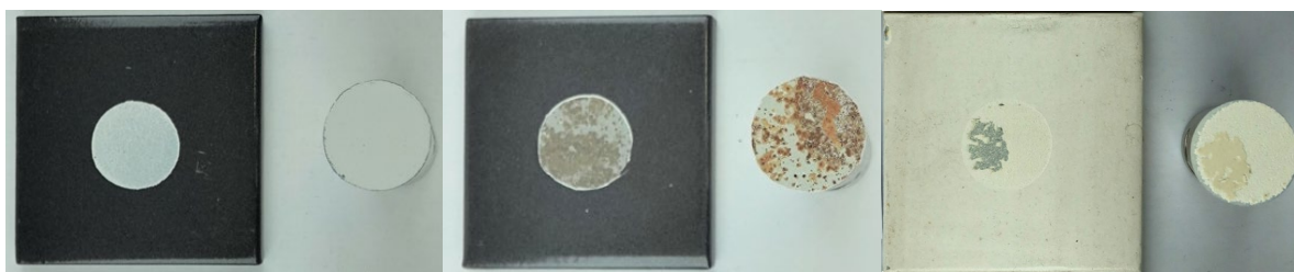
Fig. 4: Failure patterns of tear-off test specimens (cohesive failure within primer coat; adhesive failure on metal surface, mixed failure).
