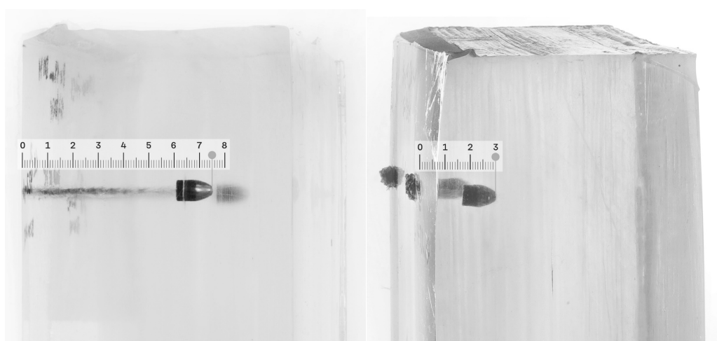
Fig. 4: left photo, regular PVB block, DoP_{Trosifol® B200} \sim 75\text{mm} , 9mm Luger, bullet velocity 423 m/s. right photo, ionoplast interlayer, DoP_{SentryGlas®} \sim 30\text{mm} , 9mm Luger, bullet velocity 422 m/s.
