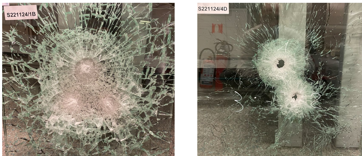
Fig. 13: (left) 2x12mm laminate after 3 shots, (right) 6x 4mm glass laminate after 2 shots.
