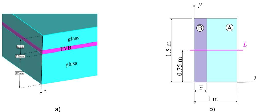
Fig. 3: (a) Considered laminated glass package and (b) model problem of the shaded panel.
