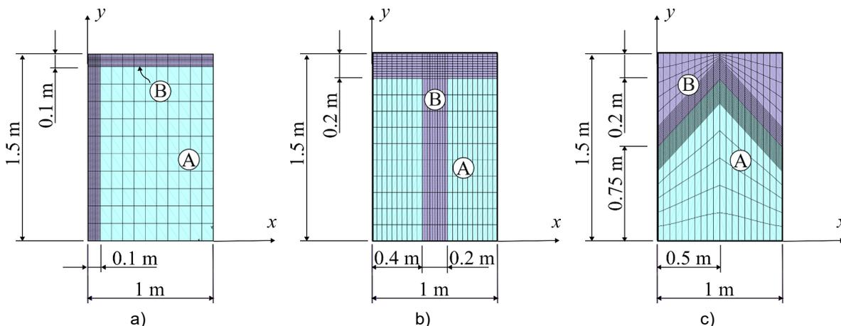
Fig. 5: Different shadow shapes considered in the study: (a) L-shaped, (b) T-shaped and (c) V-shaped.
