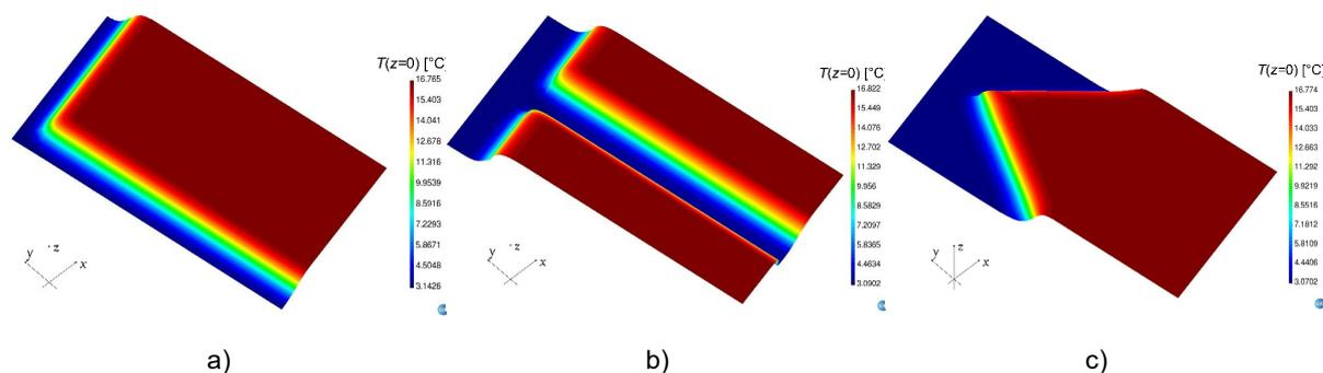
Fig. 6: Steady-state temperature distribution in correspondence of the external surfaces for (a) L-shaped, (b) T-shaped and (c) V-shaped shadows.
