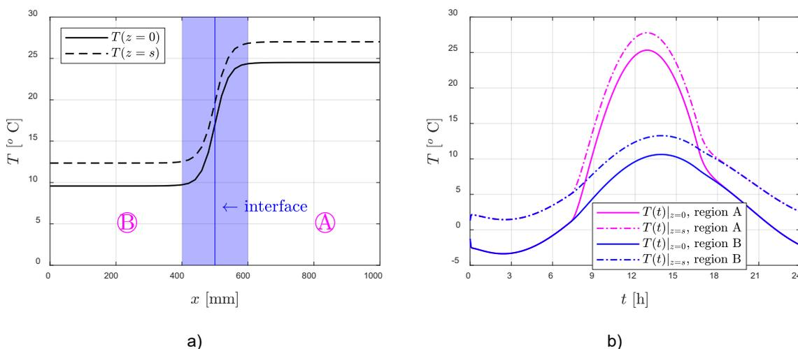
Fig. 4: (a) Spatial temperature distribution along the line L of Fig. 3(b), at 12 A.M., and (b) time evolution of the temperature on the panel surfaces.
