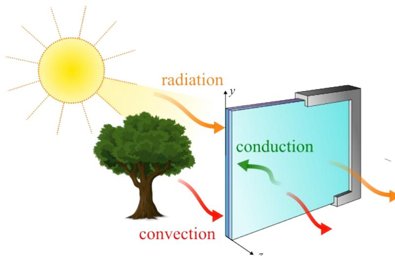
Fig. 1: Schematics of typical thermal scenario and heat exchange phenomena for a façade glazing panel.
