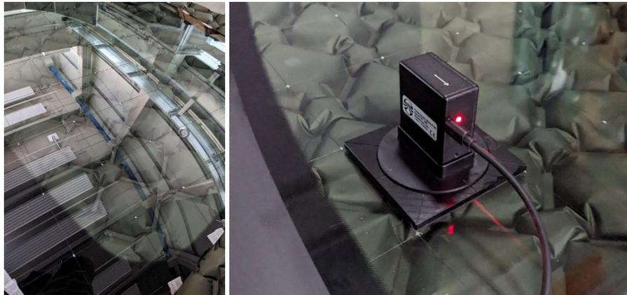
Fig. 4: Grid pattern of the windshield (left) and SCALP measurement on a curved pane (right).
