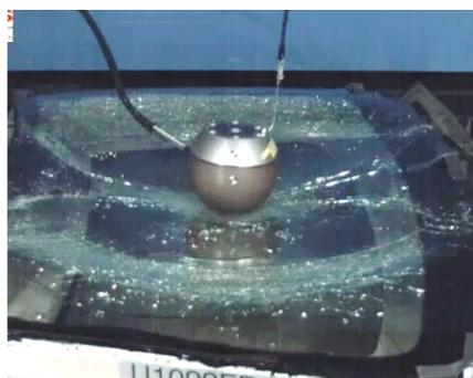
*Fig. 1: Full size impact test on windshield.*
