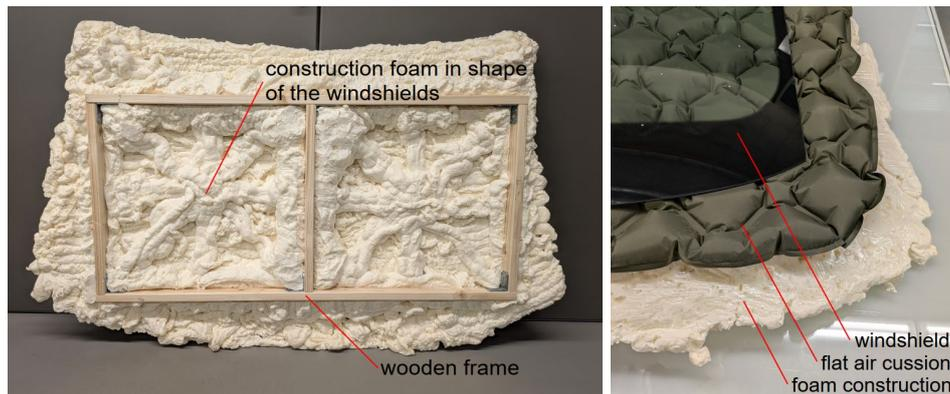
Fig. 6: Support construction made of construction foam (left), setup for SCALP measurements (right).
