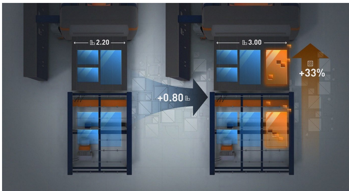
Fig. 1: Shadow Twin: Comparison of live production against the Simulated Production Layer. Increasing the oven width by 80 cm enables the processing of larger sheets or more glass per batch, leading to a 33% increase in furnace yield per charge. (A+W Glass Lab, A+W Software GmbH, 2025).
