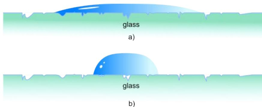
*Fig. 1: Glass surface wettability: a) better wettability and lower static contact angle b) worse wettability and bigger static contact angle.*
