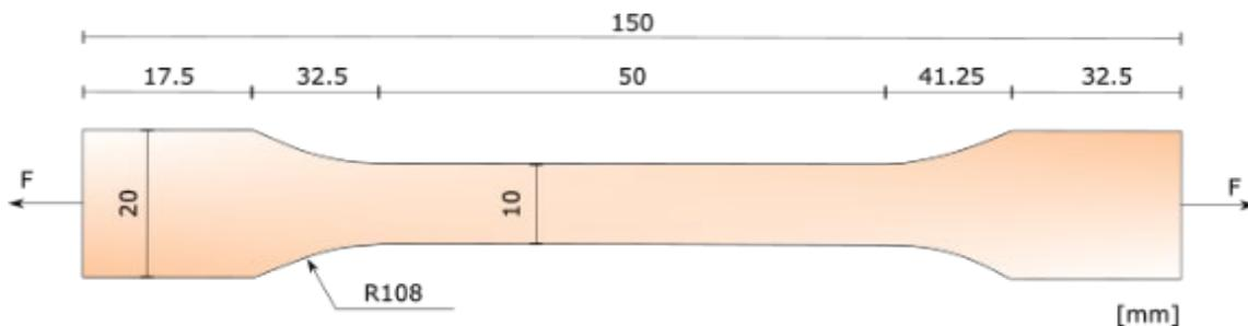
Fig. 3: Testing specimen for tensile tests.
