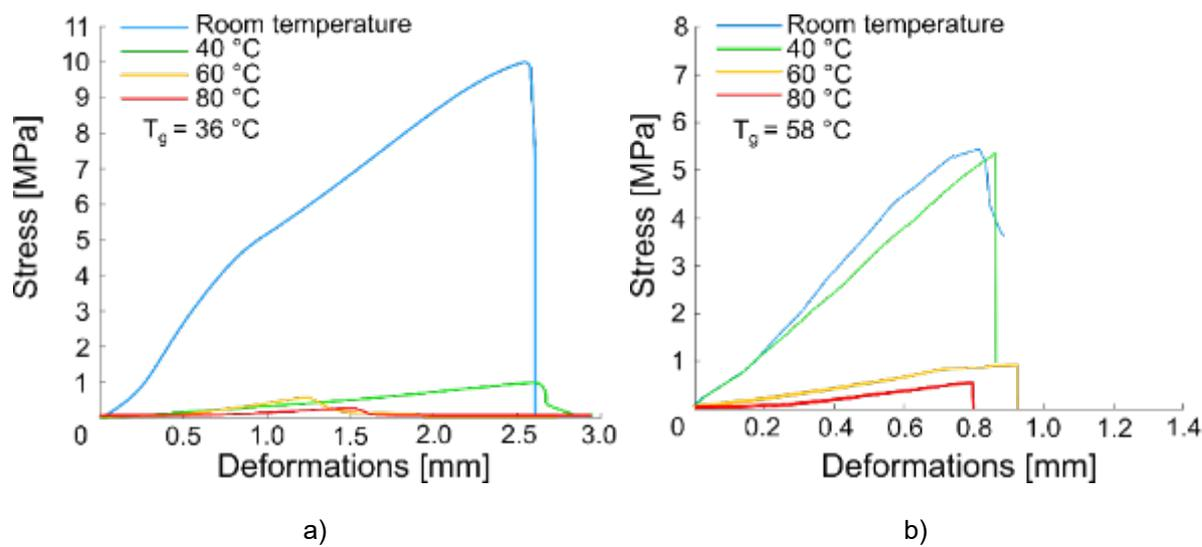
Fig. 6: Shear pilot tests a) results for Loctite® EA 9455 (Boutar , Eliášová, Tichá, & Zikmundová, 2023); b) Shear pilot tests results for Epox® G300.
