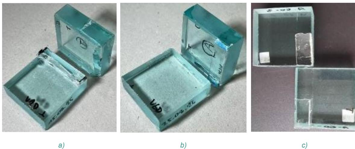
Fig. 7: Observed failure mods: a) Mixed failure; b) Adhesive failure; c) Combined failure (Boutar , Eliášová, Tichá, & Zikmundová, 2023).
