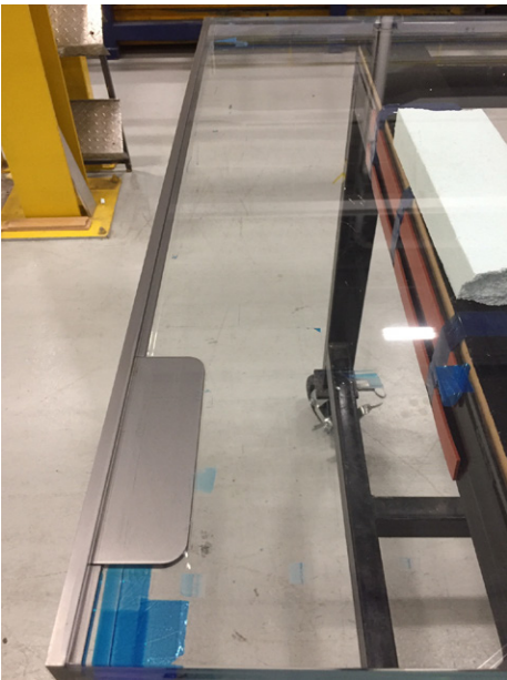
Figure 2—Titanium pivot rail embedded in the door.
