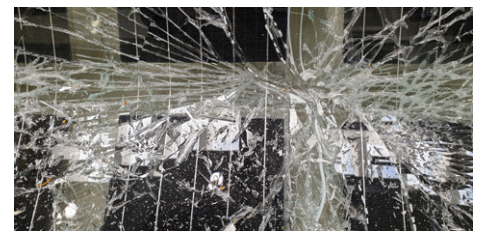
Figure 3: Test set-up and detail view of broken laminated glass with PV.
