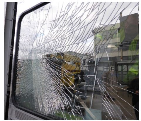
Figure 1: HVB-Tower: view of building and result of pendulum testing of facade element.
