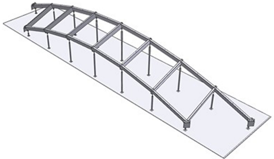
Figure 15: A green marked frame (see Figure 10) in the welding jig.
