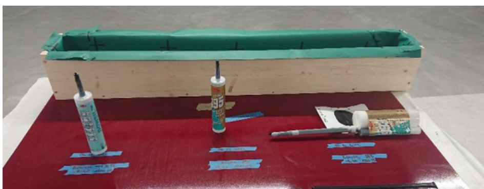
Fig. 10: DOW testing (Silicone line and water immersion test setup).
