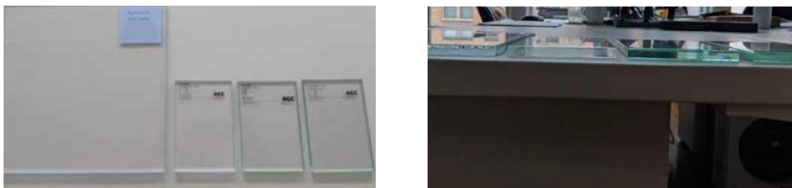
Fig. 3: Glass substrate transition from clear to low-iron at glass surface and glass edges.
