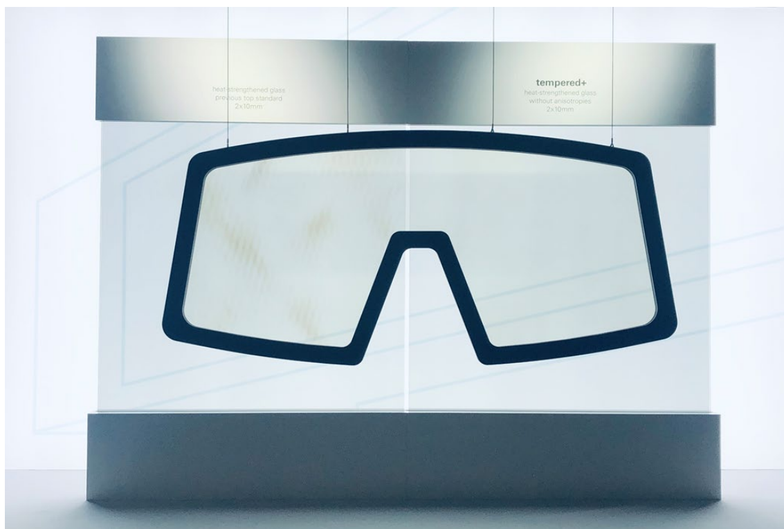
Fig. 6: Anisotropies in conventional tempered glass 2x10 mm (left) and sedak tempered+ 2x10 mm (right) (dimensions 2m x 3m).
