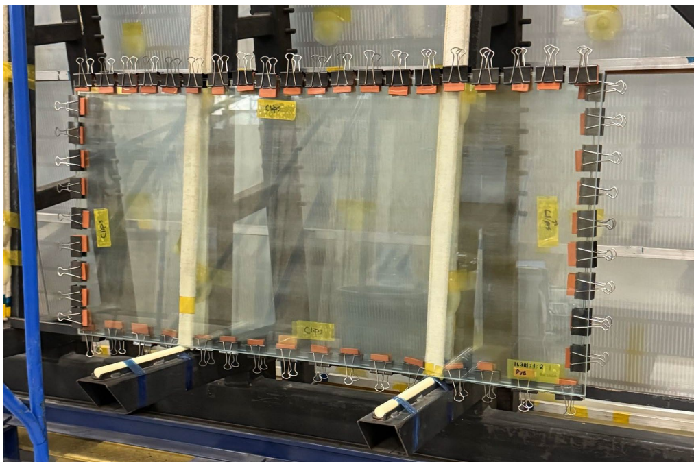
Fig. 18 - Lamination with clips to enhance distortion.
