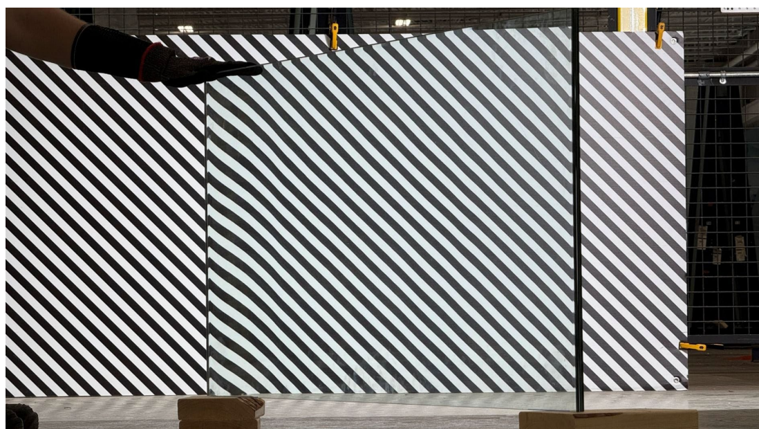
Fig. 23 - Lami 1 Zebra test at 60° we observe the same vertical distortion as with the grid test.
