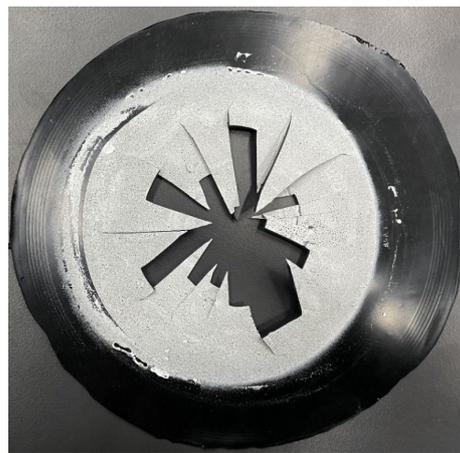
Figure 16: Failure pattern polyurethane.
