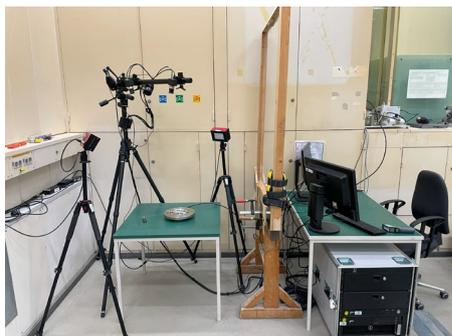
Figure 6: Test stand with DIC.
