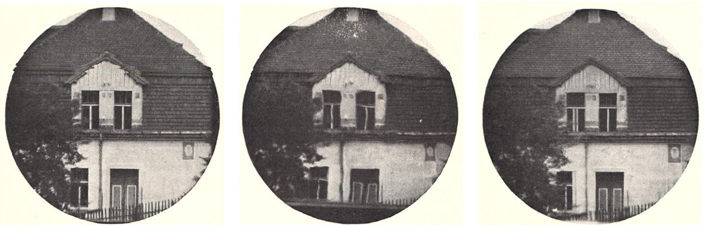
Figure 4 Views through a window with a) no window pane b) hand-blown glass and c) a pane of drawn glass (using the Fourcault method).
