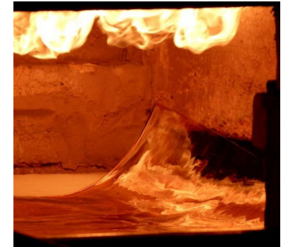
Cylindrical sleeve process. Picture: Erwin Purucker
