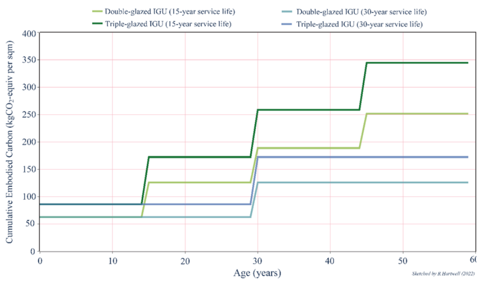
Figure 3: Assessment of the potential cumulative embodied carbon impact for an insulated glass unit. The embodied carbon of constituent materials (i.e. for glazing, spacer bar and sealant) is evaluated at 0% recycled content for all IGU systems. (Courtesy: Rebecca Hartwell).
