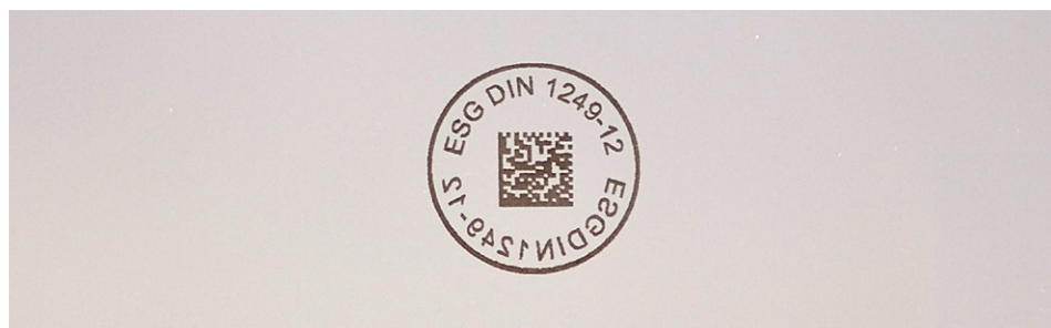
Image 4: A unique, machine-readable marking allows the glass pane to be identified at the installed situation. The marking is printed on gently without damaging the surface of the glass.
