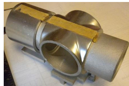
Figures 6. Typical mullion and connector interface displayed at different angles to show details. Photo courtesy of SmithGroup.
