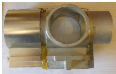
Figures 6. Typical mullion and connector interface displayed at different angles to show details. Photo courtesy of SmithGroup.
