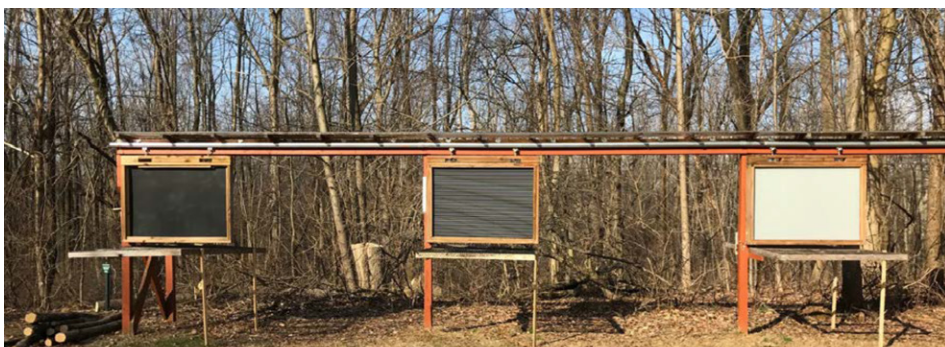
Field study to deter or prevent bird window collisions showing control on left and McGroby 95% and 100% risk reduction samples in center and right Positions.
