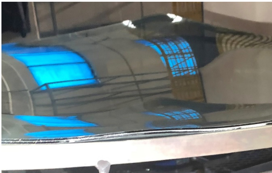
Figure 2. Shape and optical distortion issues in the windscreen after bending.
