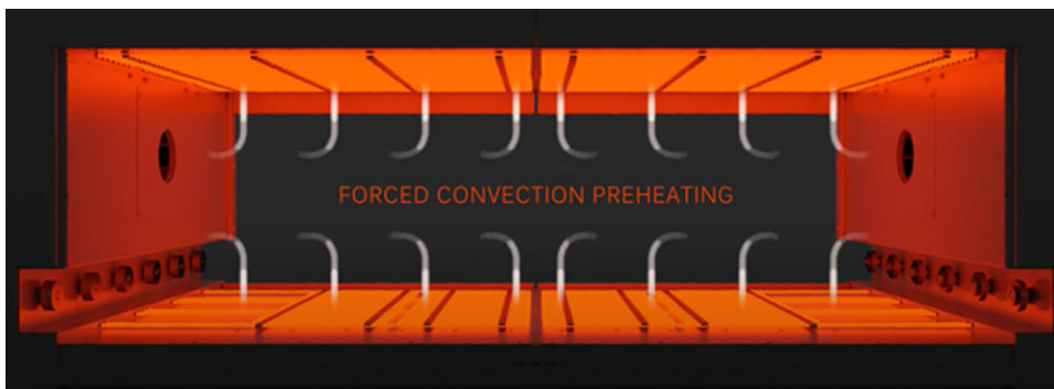
Figure 4. The illustrative image of preheating furnaces with forced convection jets.
