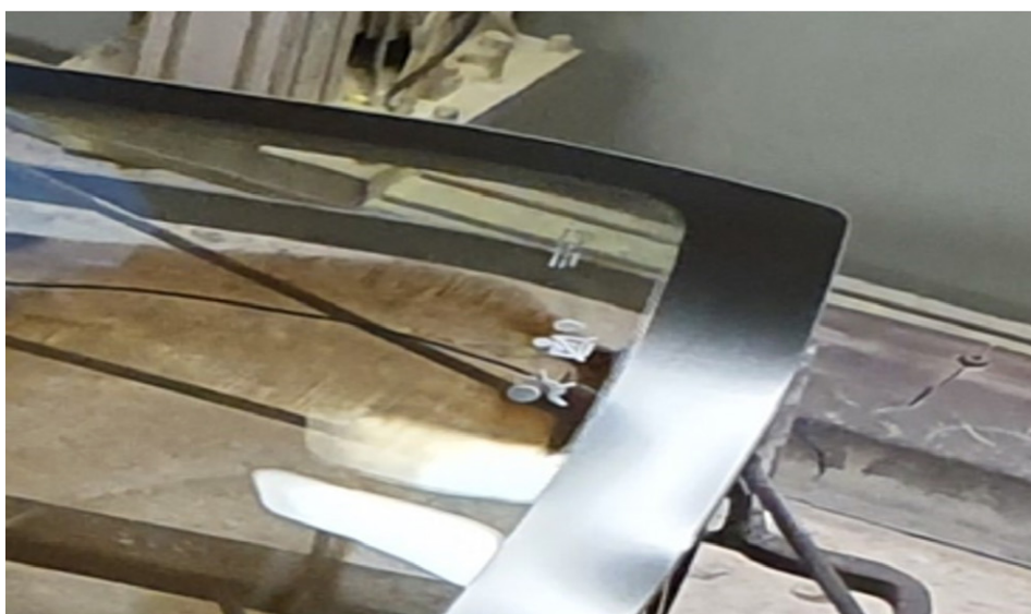
Figure 1. Windscreen with enamel edge and coating on a glass surface.
