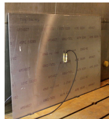
Fig. 2 Sample design 3: air injection into the bonded plate.
