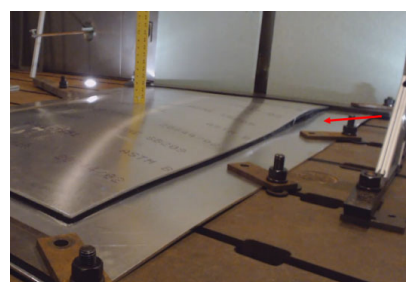
Fig. 9 Sample design 3: 20mm/40mm: failure location.
