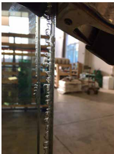
Figure 6 Edge bubbles present after autoclave
