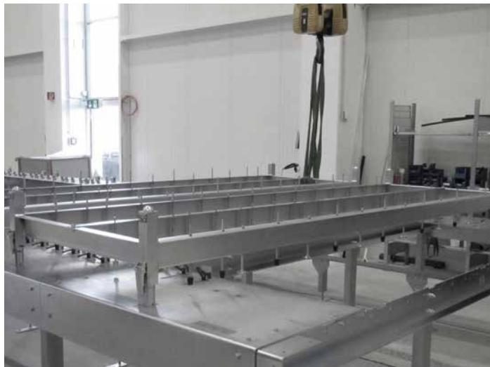
Figure 7: Bespoke lifting frames, without (left) and populated with panels (right)
