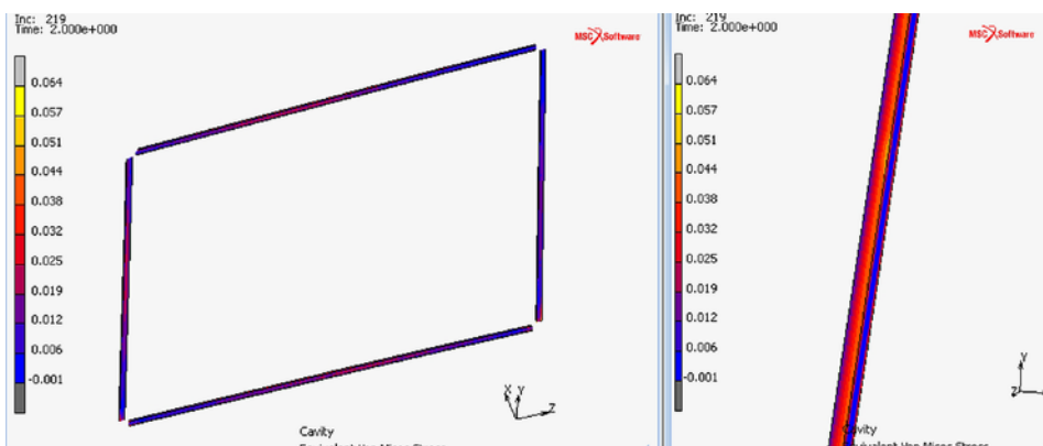
Figure 25: FE analysis stress plot of primary seal (Van Mises stress) for load case 1, excluding corner cut-out areas
