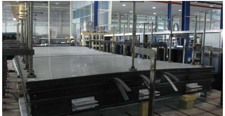
Figure 10: Free-form cold-bent structural silicone glazed unitized façade panel during glass cold-bending process, concave long edges and convex short edges
