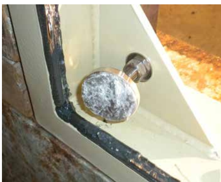
Figure 7: Glass shards adhered to the TSSA and weatherseal
