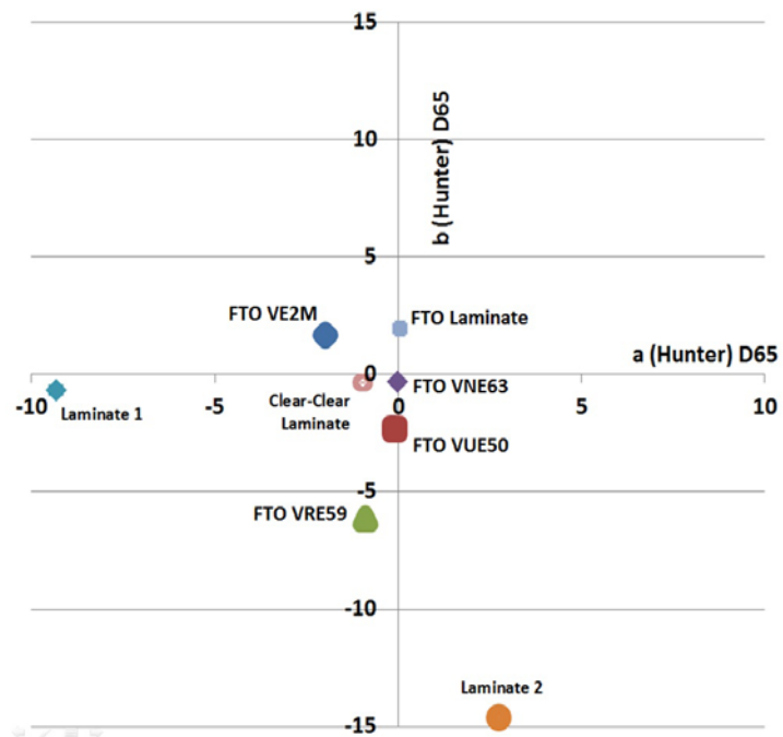
Figure 8: Interior Reflective Film-Side Measurement for Tested Products
