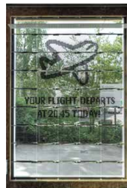
Displaying information on the SIGU with TN-modules of type 1. View from inside to outside. Phot.: G. Metzger, ILEK
