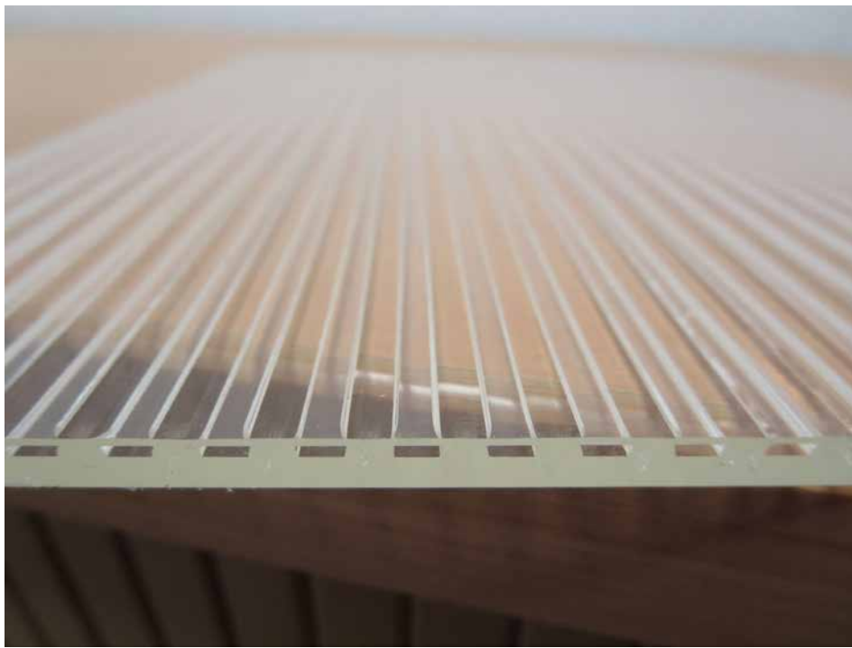
Figure 5. Side view of a composite capillary glass
