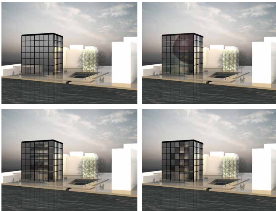
Figure 10. Application possibilities of the structured adaptive glazing in a fully glazed facade. Renderings: S. Leistner, ILEK
