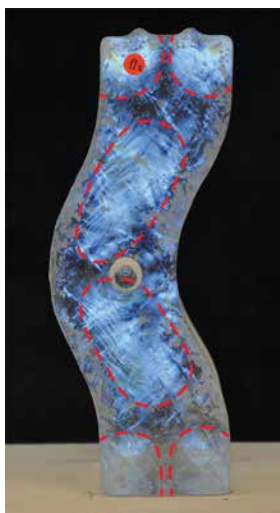
Figure 7 Typical stress zones after the kiln-casting of the bricks (Polarized image)
