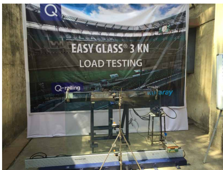
Fig. 3 Test Set for the Post Breakage Strength Test
