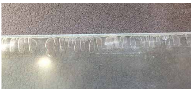
Figure 5 Edge bubbles after weathering of orientation B sample
