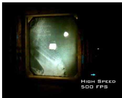
Figure 6: Glass breakage at ~4" of deflection, Frame 1, Test 1
