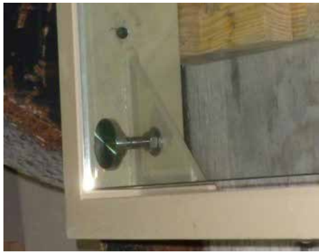
Figure 2: Glass with TSSA attachment set into
