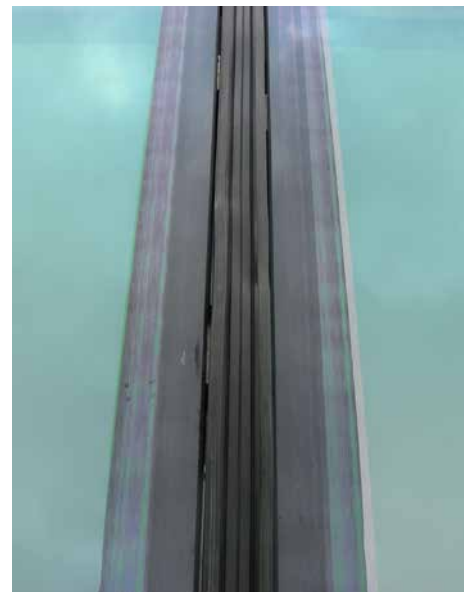
Fig. 2: Glass with edge deletion by grinding, showing typical grinding marks
