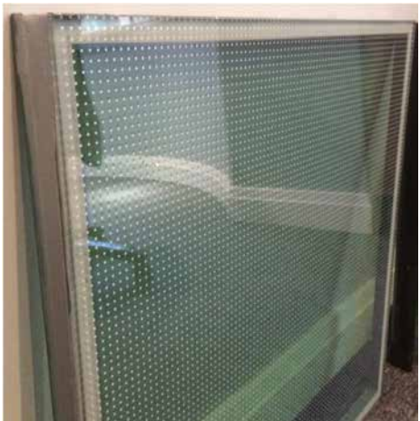
Figure 7.2: Glass Sample of 7,5% fritting, 2 mm white dots + grey edge Stopray Ultraselect 50. Interpane. (Denton Corker Marshall, London)
