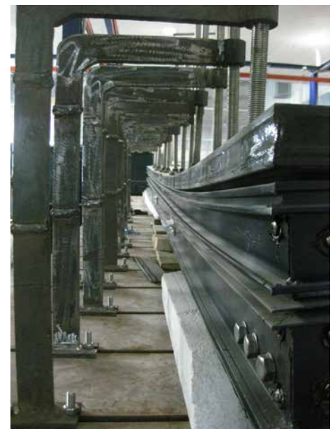
Figure 11: Free-form cold-bent structural silicone glazed unitized façade panel during glass cold-bending process, concave long edge
