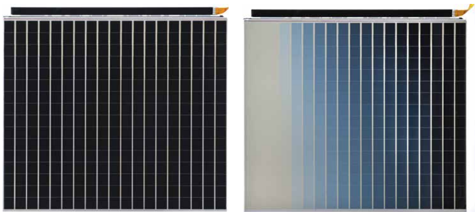
Figure 4. TN-modul type 2: all pixels in "on" state (left), graded transparency (right)
