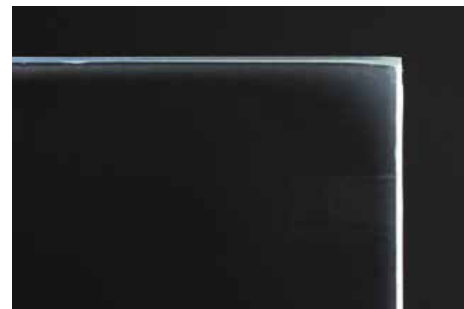
Figure 9 Standard PVB after 1,000 hours in the salt spray test
