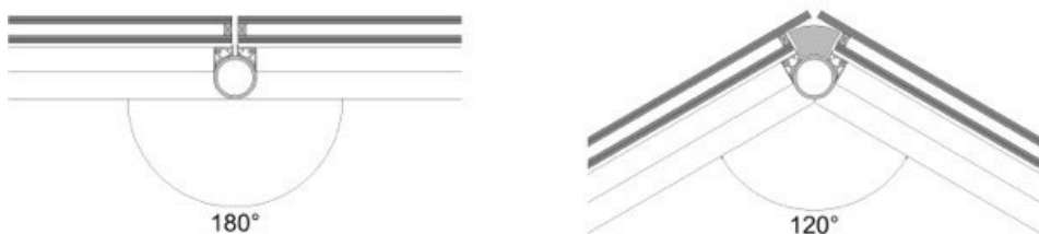
Figure 4: The length of the stepped glazing is dependent on the angles of the design geometry
