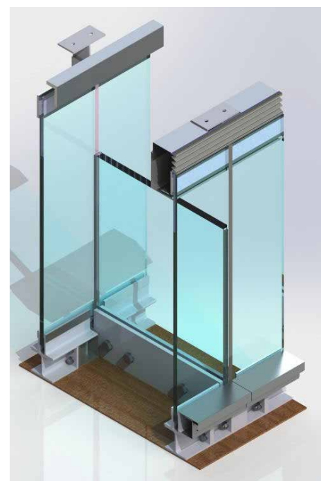
Figure 2. 3D Image for small visual mock up to show the double skin of glazing
