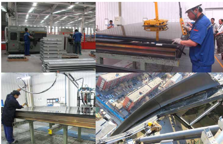
Figure 23 Factory fabrication and Site Assembly
