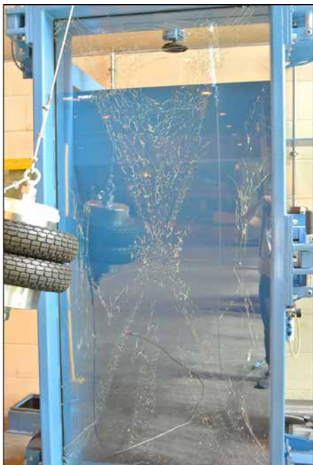
Figure 3. Pendulum test according to DIN EN 12600 on laminated glasses with EVA interlayer. Result for low crosslinking (left) and high crosslinking (right)
