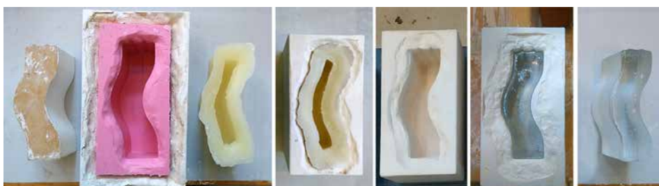
Figure 2 Production steps from MDF mould to final glass model
