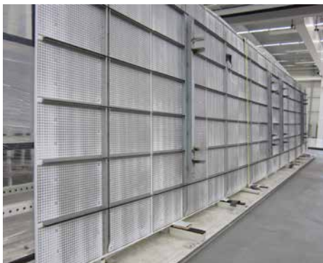
Figure 4: 15x3m composite panel viewed from the panel side.
