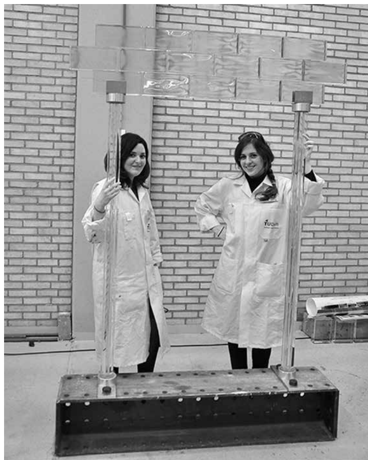
Left: Realized 1.5m long prototypes of the bundled column by the authors
