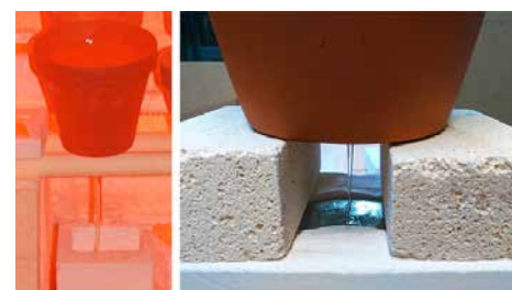
Figure 5 Glass flowing from the flowerpot down to the mould
