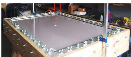
Figure 1. Uniform Lateral Load Test Machine.
