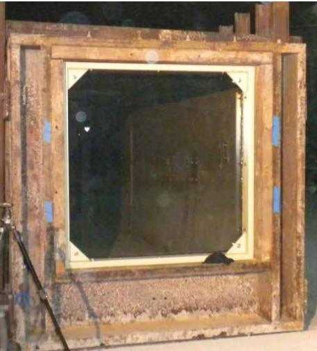
Figure 4: Frame and glazing installed into the shock tube
