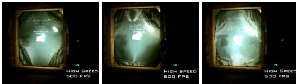
Figure 8 (A) (B) (C): Glass Failure at test 4, 6, and 9
