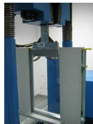
Figure 2. Pull-out test setup
