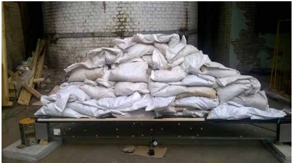
Fig.16 fully loaded mock up, taking 3 tonnes of sand bags.
