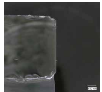
Figure 7 Microscopic view of failure origin [6]
