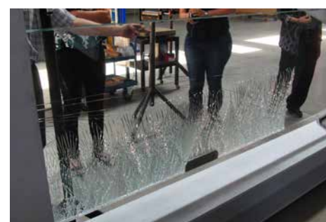
Figure 3. Glass fin after the first failure
