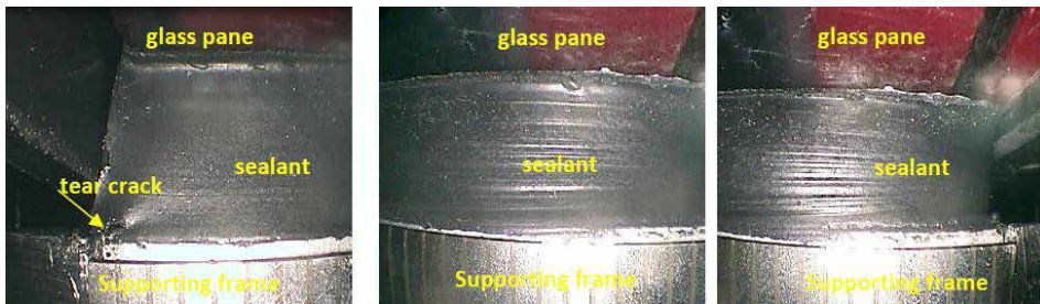
Figure 10: Visual investigation of system bond after simulated 50 years of use (here: 2 nd generation SSG)
