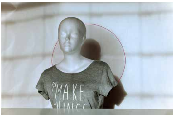
Figure 8. Shadow caused by spot on the glazing to prevent glare effect on occupant. Phot.: G. Metzger, ILEK
