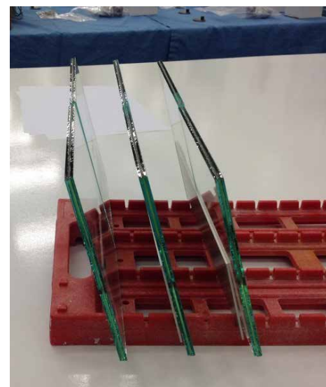
Figure 4: Laminated glass in exposure rack for Salt Fog testing
