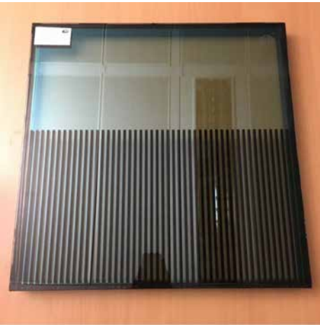
Figure 7.1: Glass Sample of 5% fritting, 5 mm vertical black stripes. Guardian SNX 50/23. (Denton Corker Marshall, London)
