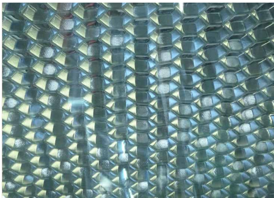
Fig 3 Perforated honeycomb bonded to glass
